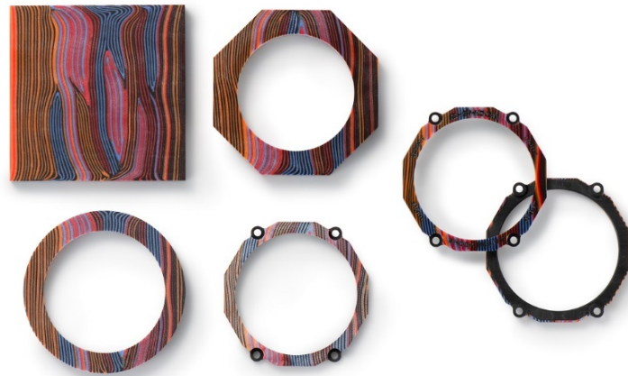
Steps in making the multicolor carbon bezel
