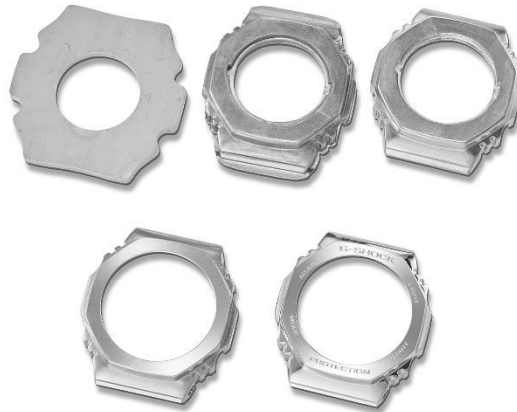
Bezel forging process
